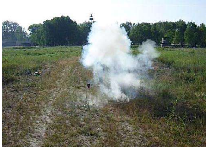
Figure 3. The shape and size of the cloud active substance immediately after the tear action item has been activated
