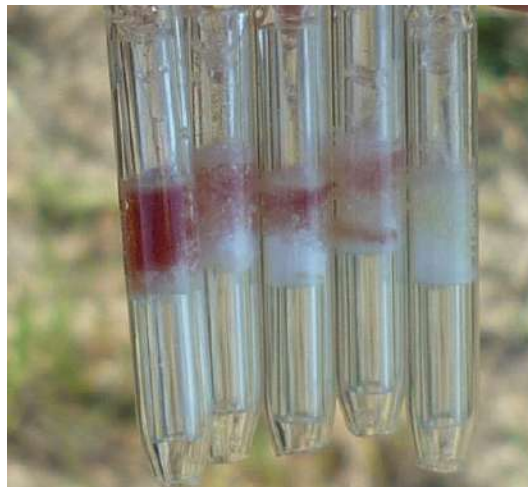
Figure 4. Change the color of the indicator tubes filler on CS (concentration \geq 5 \text{ mg/m}^3 )
